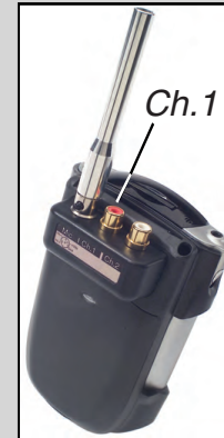
Step 3- Connect to Ch.1 Line Input RCA connector
