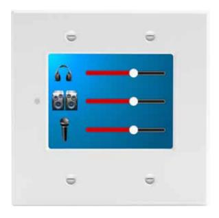
The iTC-1 is a programmable 3.5" touch-panel wall control for custom OEM applications. The iTC-1 has a 1/4 VGA configurable full gui interface that can be defined to fit nearly any application. The iTC-1 fits into a standard 2-gang wall box or re-work box, and is powered by 24 volts DC over CAT5 cable using RS232 or RS485 control strings up to 1,000 feet. The iTC-1 comes with gui design and control software.
